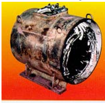
Figure 2: Stator that has been through the burnout process
