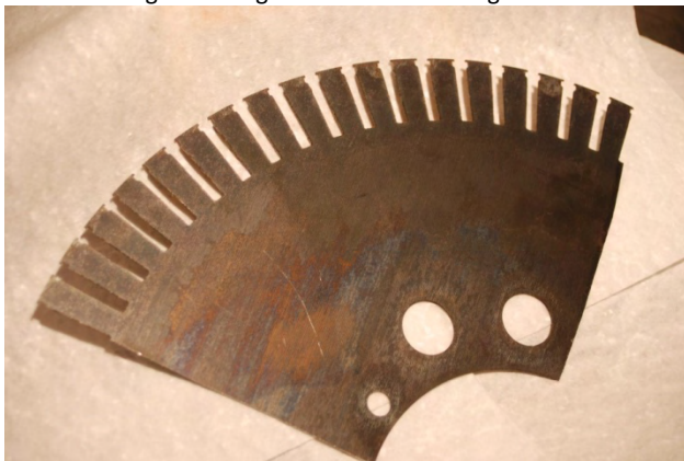
Figure 1: Degraded Lamination Segment
